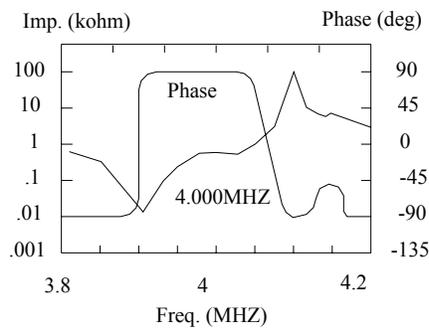
Fig. 3 Impedance vs. phase of a 4.000 MHz ceramic resonator.
